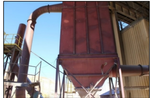
Fig. 8 Dust collector has inwardly converging walls
