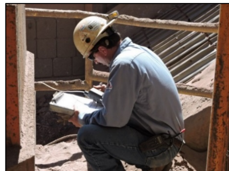
Fig. 35 Taking pre-entry monitor readings
