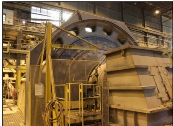
Fig. 2 A ball mill is a confined space
