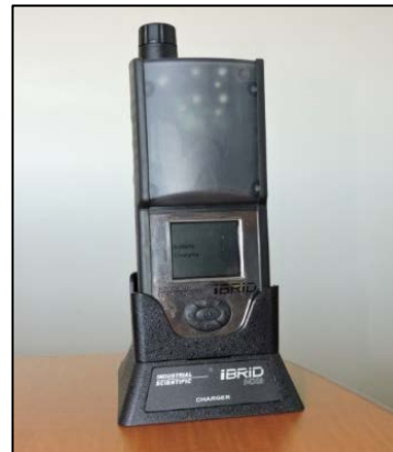
Fig. 33 Example of an air monitor
