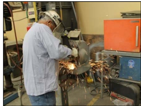
Fig. 10 Using a stationary grinder
