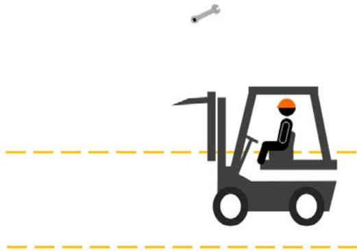
Fig. 2.13 Toe boards prevent these types of incidents
