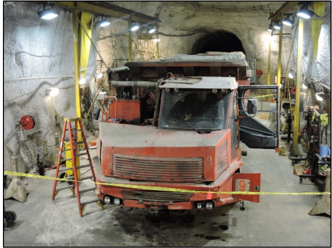
Fig. 1.2 Flagging a work area
