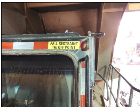
Fig. 17 Tie-off point on a haul truck
