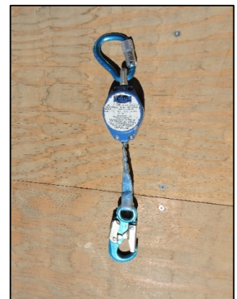
Fig. 37 Example of an SRL
