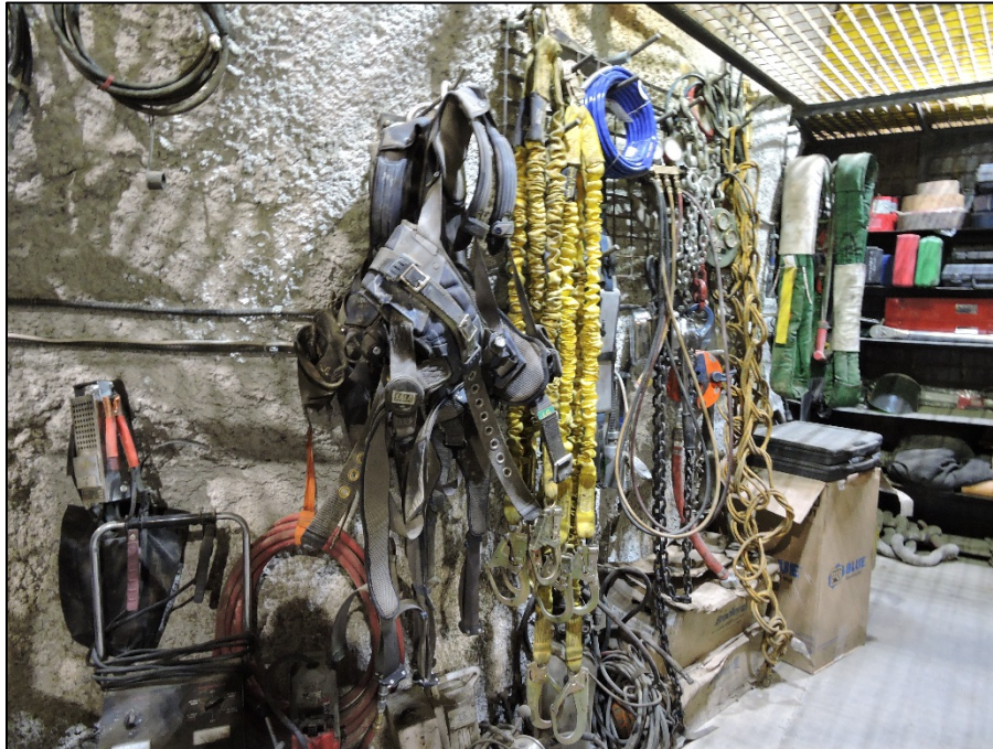
Fig. 48 Proper storage of equipment
