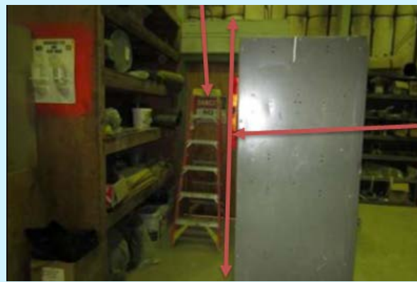
Fig. 2 Employee used 6ft ladder to reach up 8ft 5in
