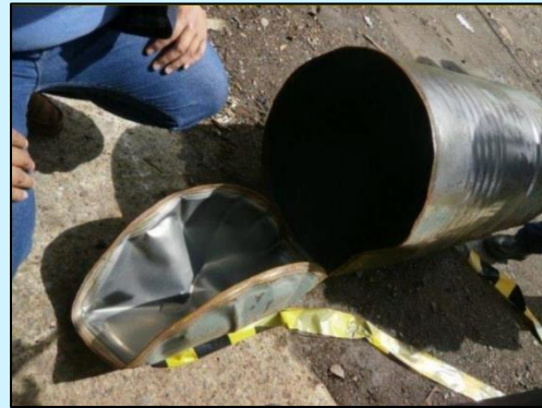
Figure 7.5 Drum failure after ignition from (PFE) above.
