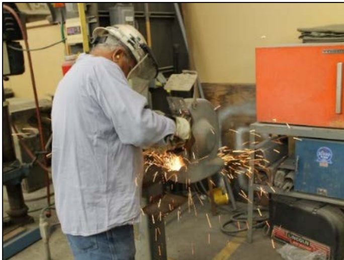
Fig. 3.3 Using a stationary grinder.
