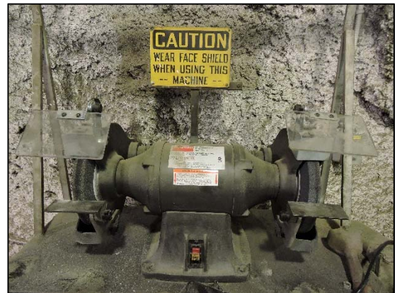
Fig. 2.17 Using a stationary grinder
