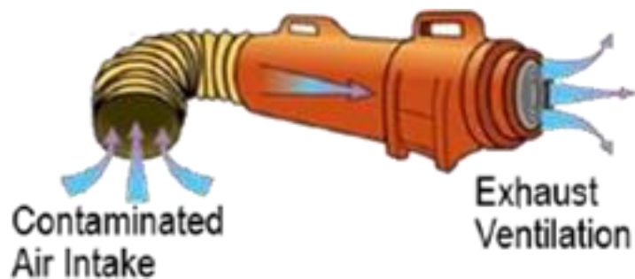
Figure 2.8: Local exhaust ventilation diagram
