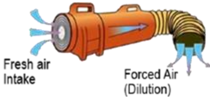
Figure 2.9: Forced air ventilation diagram
