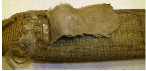
Figure 3.35: Damaged illegible capacity tag
