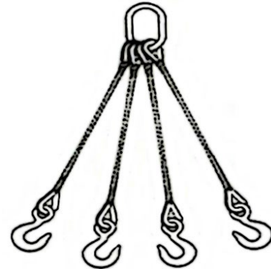
Figure 4.21: Four Leg Bridle Hitch
