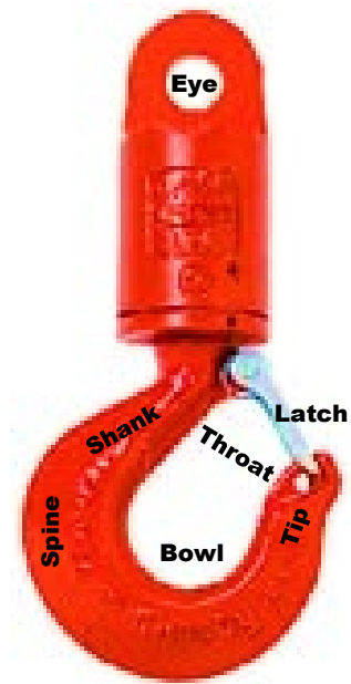
Figure 2.10: Hook Components
