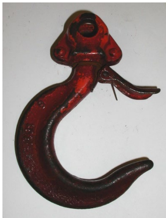
Figure 2.11: Stretched throat opening
