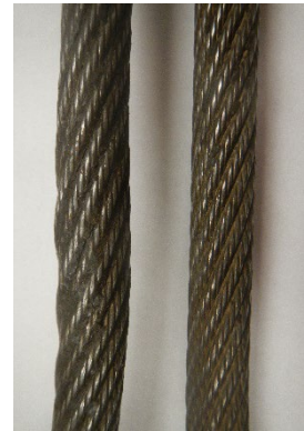
Figure 3.14: Examples of Right Hand Lay Rope
