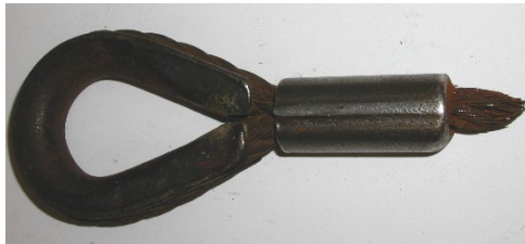
Figure 3.18: Rope failure at fitting due to corrosion and broken wires
