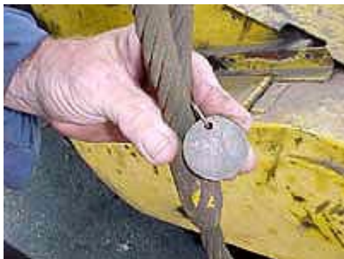
Figure 3.19: Dry brown rope which needs lubrication
