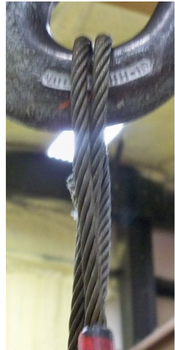
Figure 2.13: Incorrect Placing of Slings
