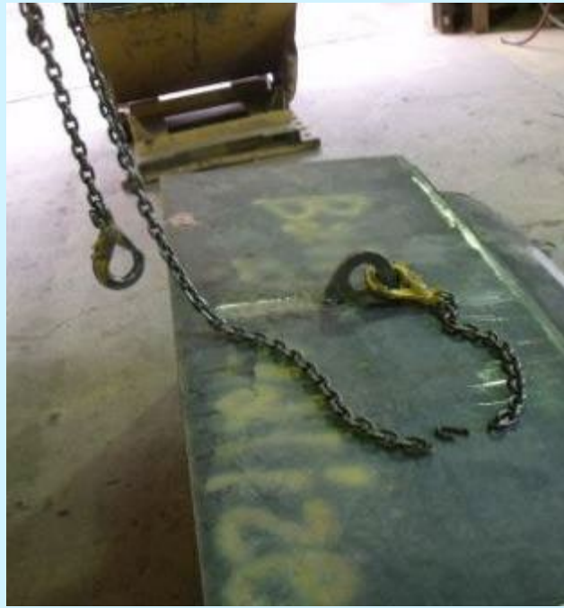
Figure 1.5: Broken Sling Leg
