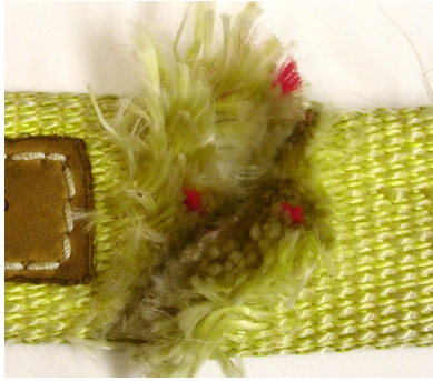
Figure 3.38: Exposed Red Yarns
