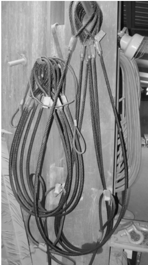
Figure 3.28: Good Wire Rope Sling Storage
