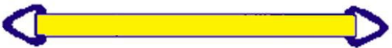
Figure 3.30: Triangle and Triangle has hardware on each end for use in a basket or vertical hitch.
