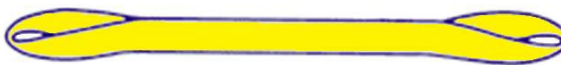
Figure 3.32: Twisted Eye and Eye has eyes turned at a right angle to sling body, forming a superior choker hitch, allowing a better fit on a hook in a basket hitch.
