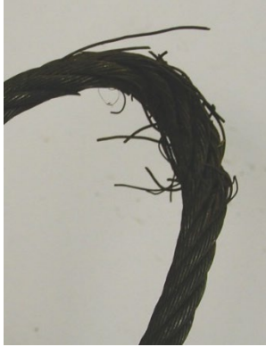
Figure 3.20: Multiple Broken Wires
