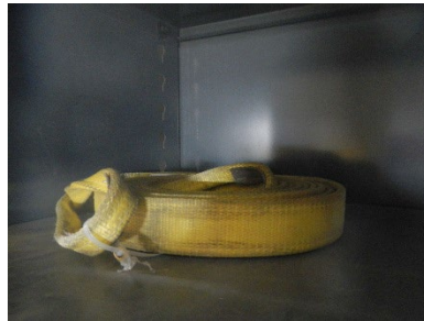
Figure 3.49: Web slings can be rolled for storage
