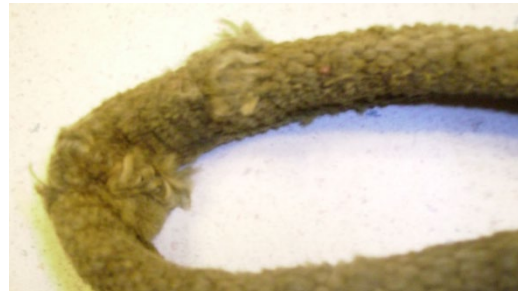
Figure 3.46: Chaffed Lifting Eye
