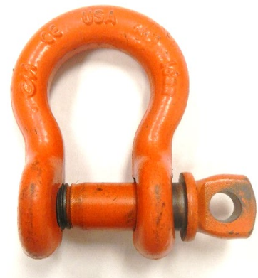
Figure 2.29: Incorrect Rigging of a Screw Pin Shackle (pin not seated)
