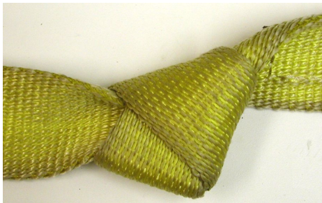
Figure 3.40: Knots in Sling
