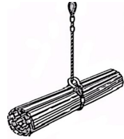
Figure 4.12: Single Wrap Choker
