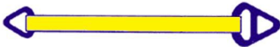
Figure 3.29: Triangle and Choker has hardware on each end - the most effective choker hitch.
