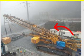
Super lift mast collapsed backward over car body.
