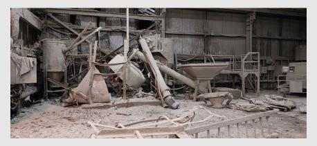
Blow pot and cement transfer facilities damaged by explosion.
