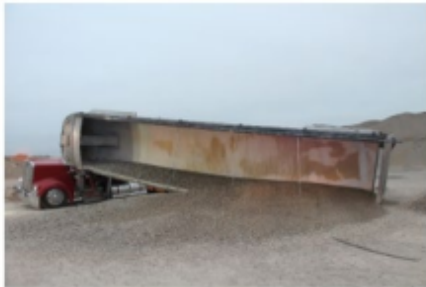
Photograph: Trailer tipped over onto cab of tractor.
