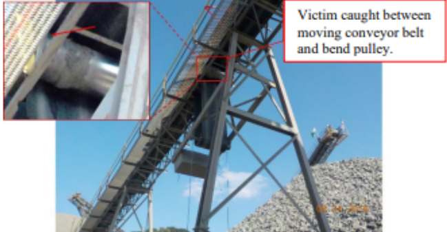
A miner suffered fatal injuries in 2018 when he was entangled in a conveyor's take-up assembly. He was working from an elevated aerial lift cleaning buildup from a bend pulley while it was operating.
