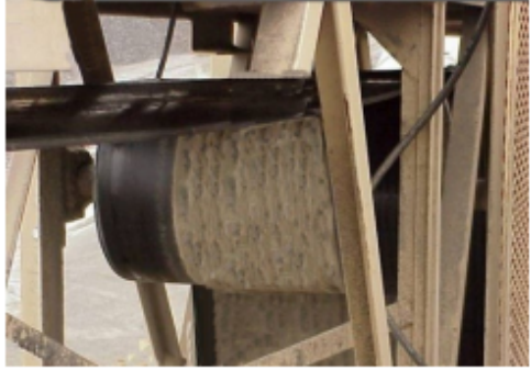
This photo shows buildup on a bend pulley. In 2024 a miner lost a thumb when he removed a guard and began to clean a rotating bend pulley with a 15-inch-long pry bar.
