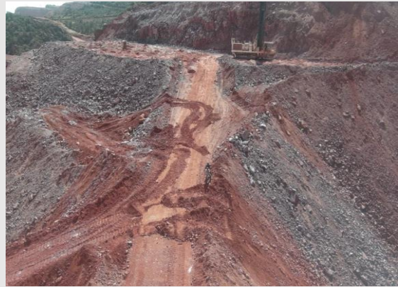
Water truck tire marks on ramp and impacted berm
