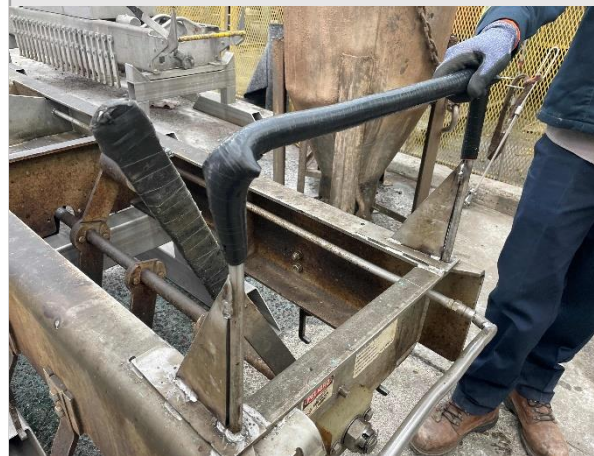
Handle with replaced insulation
