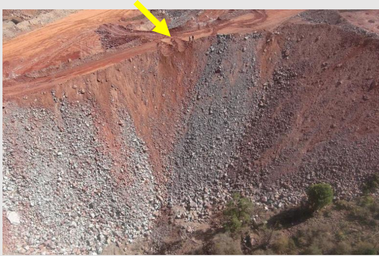
Water truck tire marks on ramp and impacted berm
