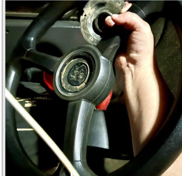
Detached haul truck steering wheel.
