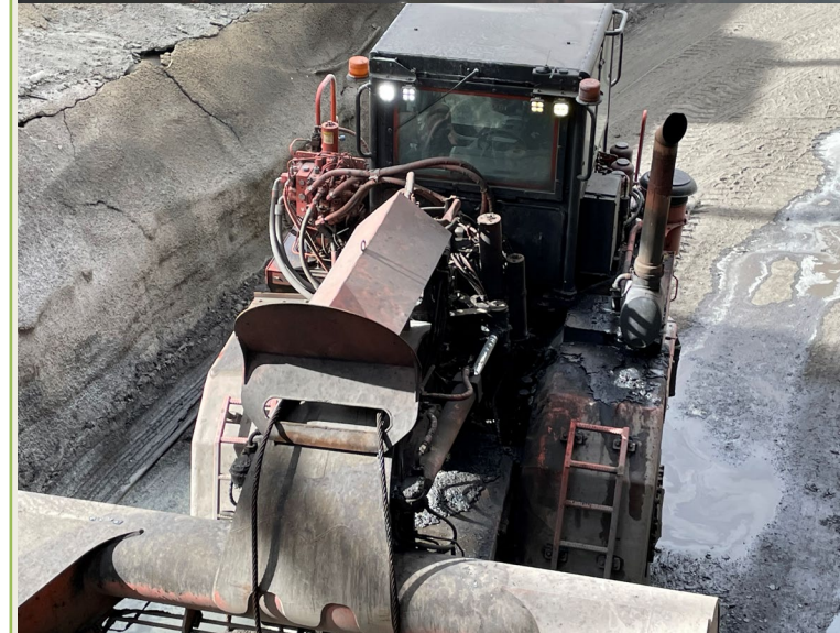
Damage to the slag hauler.
