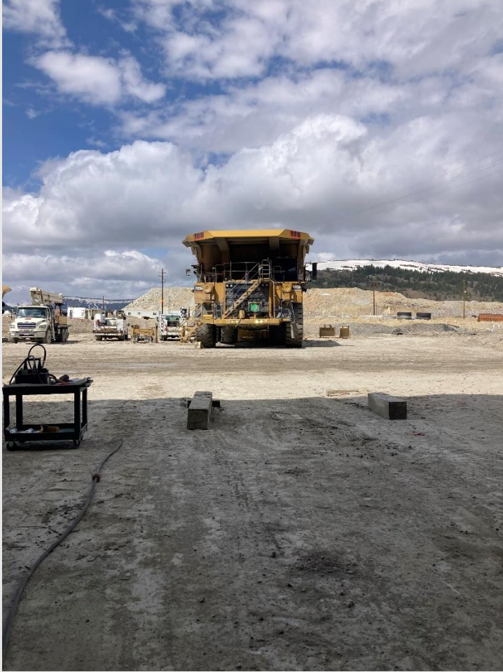
A view of the haul truck after it rolled off the wood planks and crossed the road in reverse before coming to a stop against a berm.
