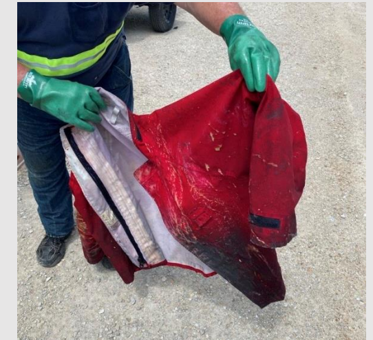
Contractor suit following acid exposure.
