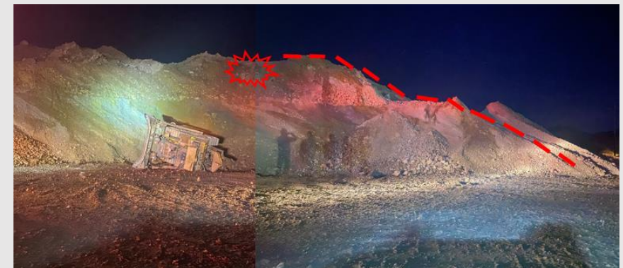
• Trajectory of the tractor, to the point where it slid and rolled down an 8-meter bank.
