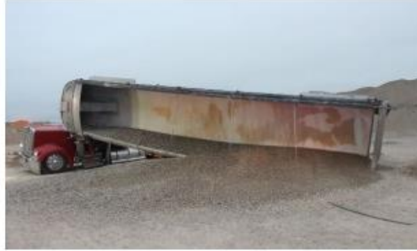
A truck driver died when his trailer tipped over onto the cab of the tractor. The driver was dumping part of the load of gravel from the trailer.
