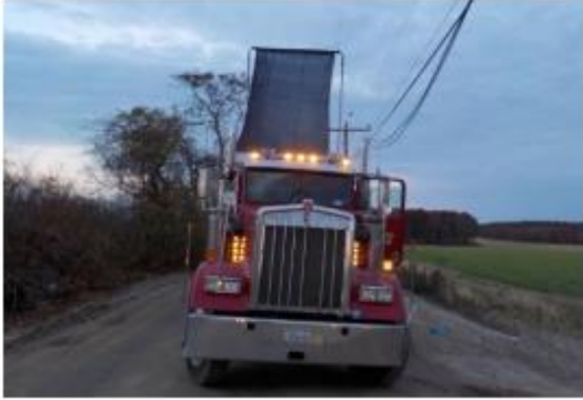
A truck driver was electrocuted when he tried to re-enter the truck's cab while the trailer's tarping mechanism was in contact with an energized overhead high-voltage power line.
