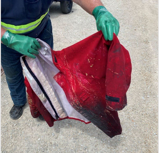
Contractor suit following acid exposure.
