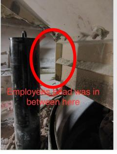
Pinch Point – Hydraulic ram and feeder
