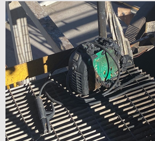
Burned welding machine.
