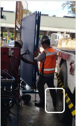
• Incident reenactment. Position of employee's right foot and the welding screen. The lowboy was moving 5km/h (3 mph).
