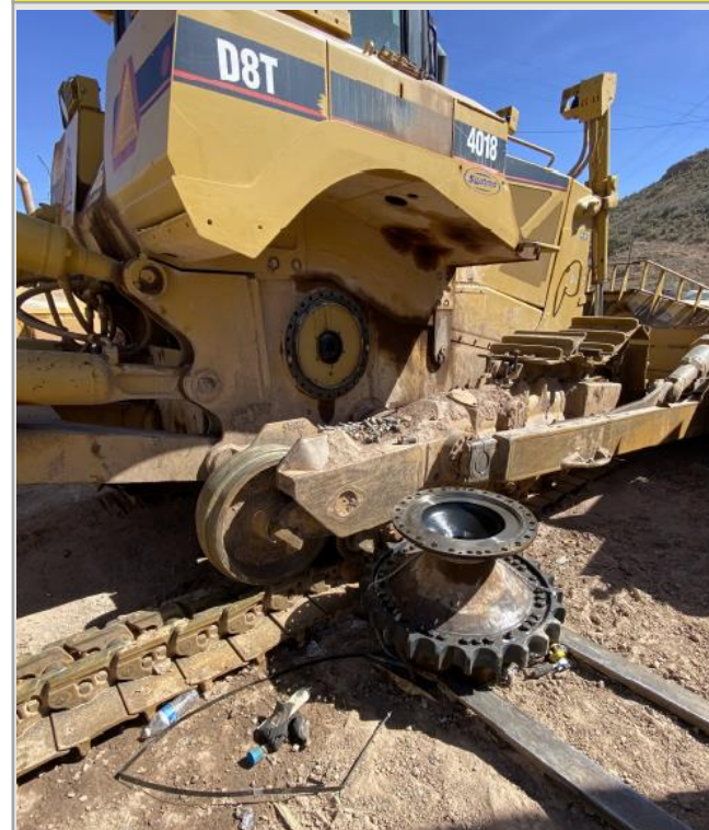
Final resting place of final drive after rotating off the forklift
