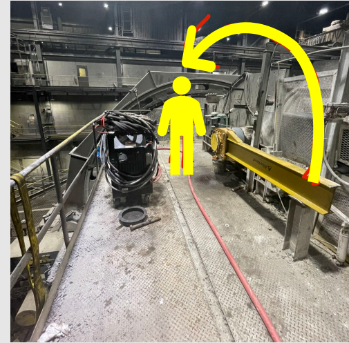
Employee location and direction of travel of the holdback device
