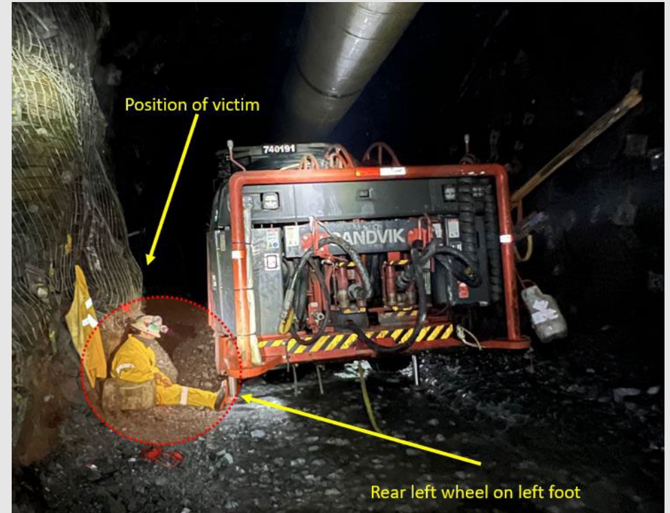
Position of offsider and Jumbo drill when backing up
