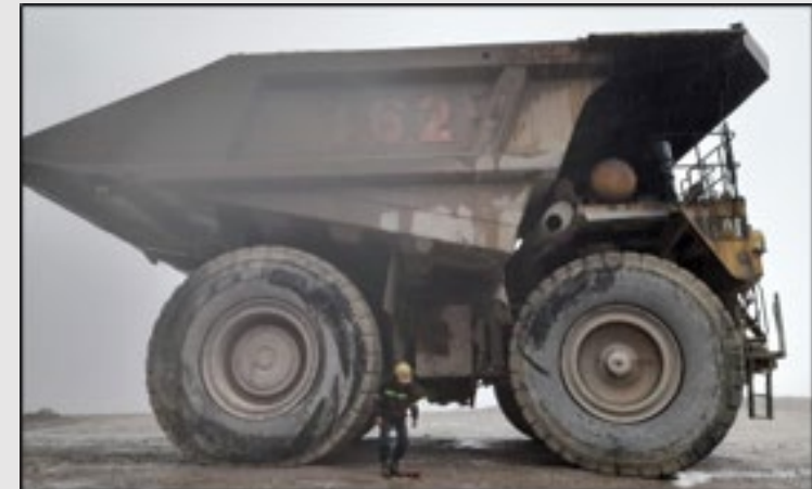
Skid marks visible on outer right wheel of haul truck
