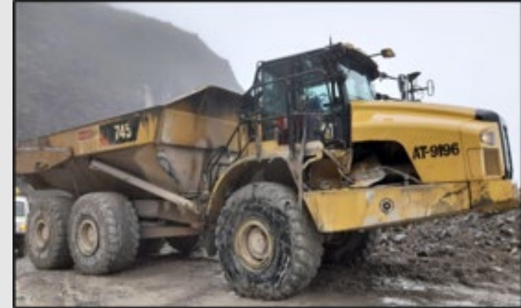
Damage to the right front side of the articulated truck
