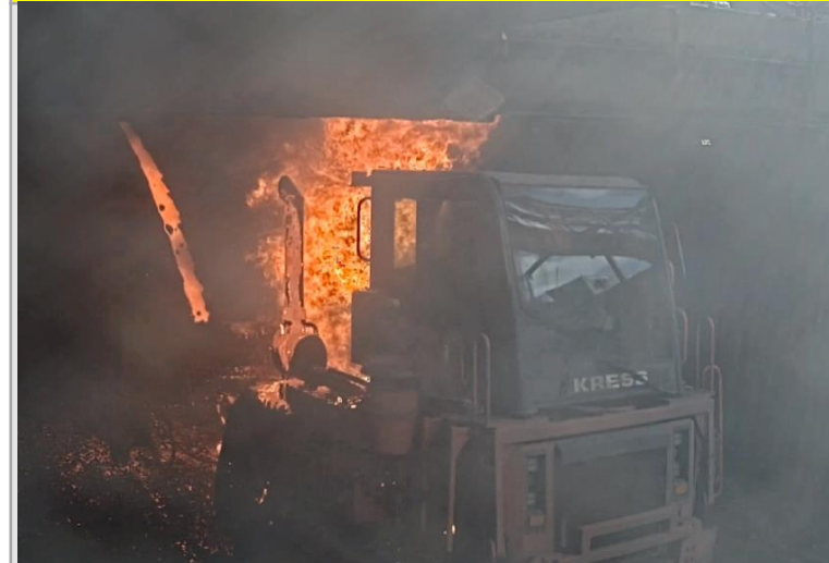
The slag hauler caught fire after molten material flowed onto it.
