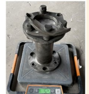
Shaft with broken-off coupler
