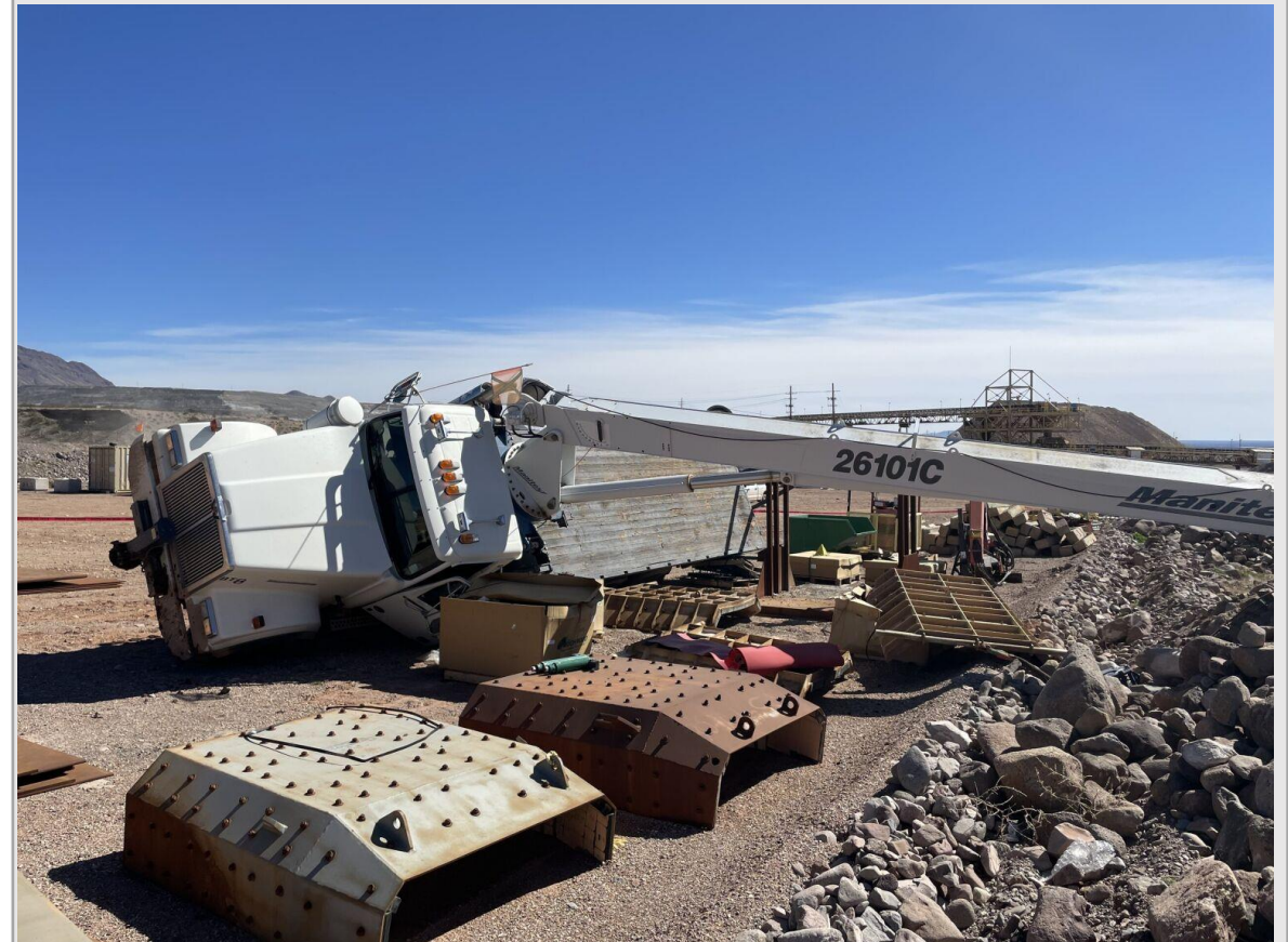
The boom truck tipped onto the driver's side when the load swung.
