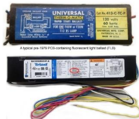
A typical non-PCB containing fluorescent light ballast. The ballast has a "No PCBs" marking on the top of the ballast and the text "electronic ballast". Only magnetic fluorescent light ballasts contained PCBs.
