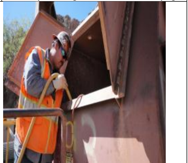
Remote unplugging from a safe location above or to the side and exterior end of the chute opening.
