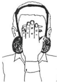
Positive Pressure Test (try to blow air out)
