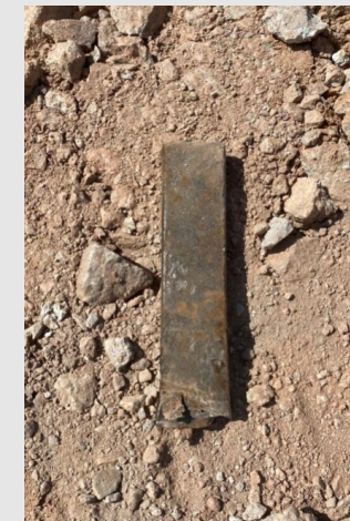
Steel wedge (3 lbs) landed 51ft from the drill.
