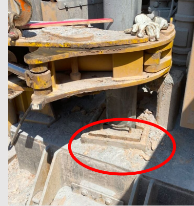
Position where steel wedge was installed and later dislodged.
