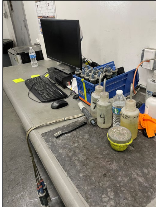
Food consumption area next to chemicals. Not cited, but could have been. 56.200014
