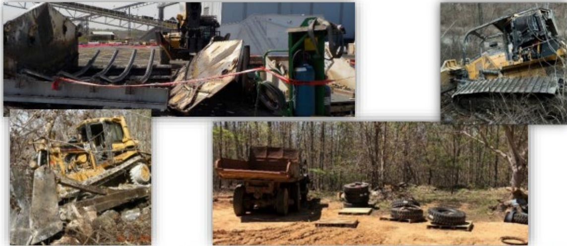
(Left to Right) Shaker screen disassembly. Bulldozer rolled down an embankment. Locking Ring dislodged from truck wheel. Bulldozer rolled down an embankment.
