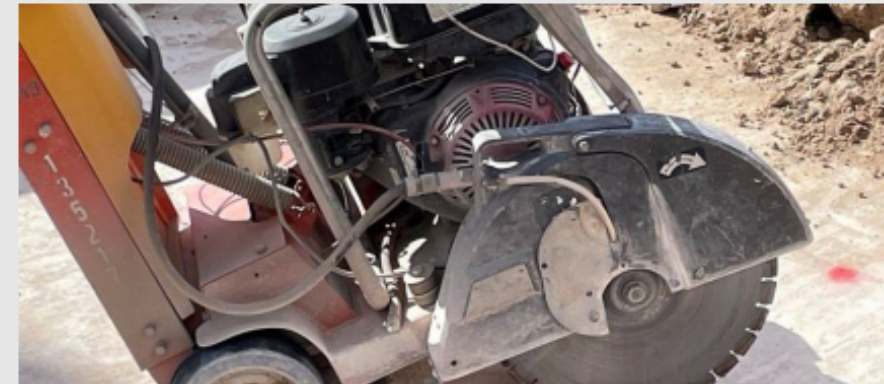
Saw used to make cut into concrete
