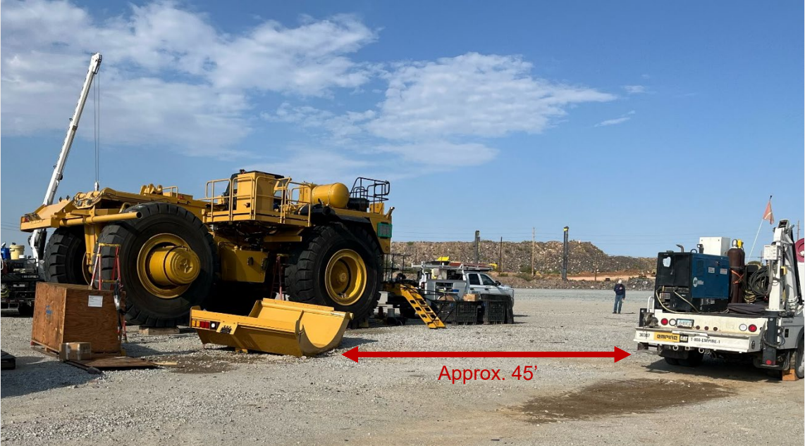
Lowboy fender after falling to ground (approximately 45 feet to crew members gathered at truck).
