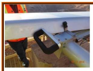
Deteriorated rubber cushion on bracket -Cover normally held in place by brackets, however was dislodged and pushed out of alignment as radar moved along track.
