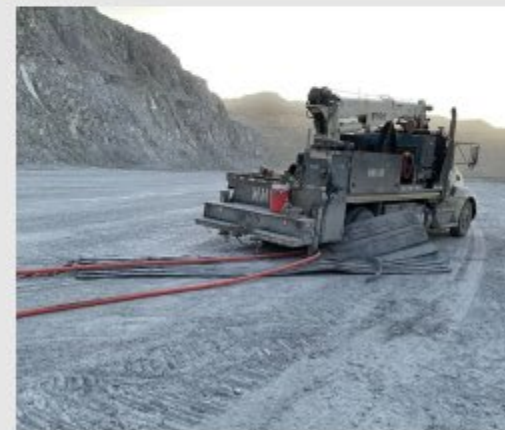
Service truck with cable and mat caught on the outrigger.
