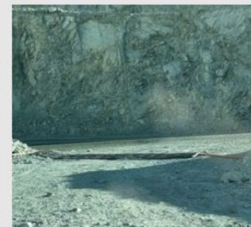
Cable and crossover mat before contact with truck.
