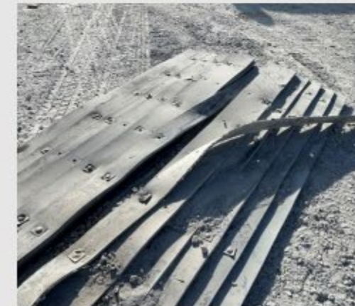
Condition of the crossover mat after contact with truck.
