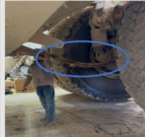
The retaining cable attached from truck bed to haul truck frame
