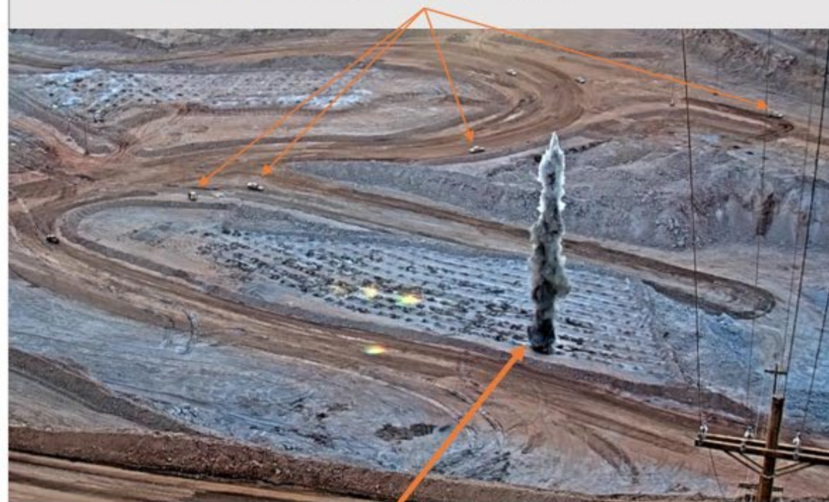
Unplanned hole ignition.
