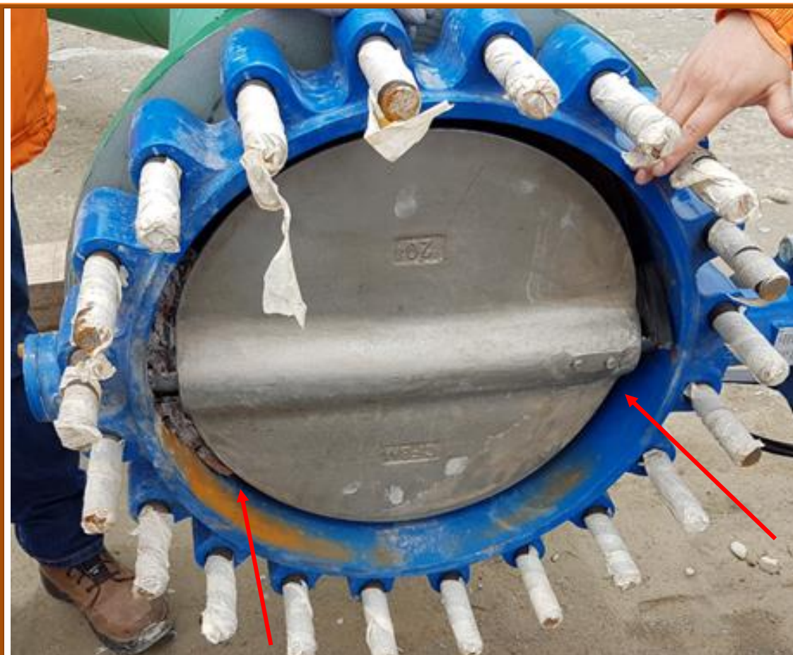
Figure 1 Las Bambas valve involved in the incident. The rubber seat material failed and broke free, leaving a gap between the metal valve body and the butterfly disk.
