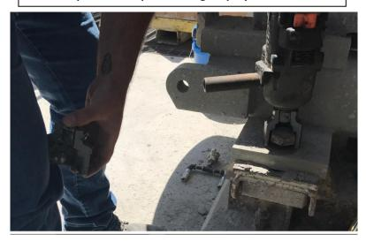
Photos showing the broken socket after the accident and a red keeper ring which should have been used as a best practice.
