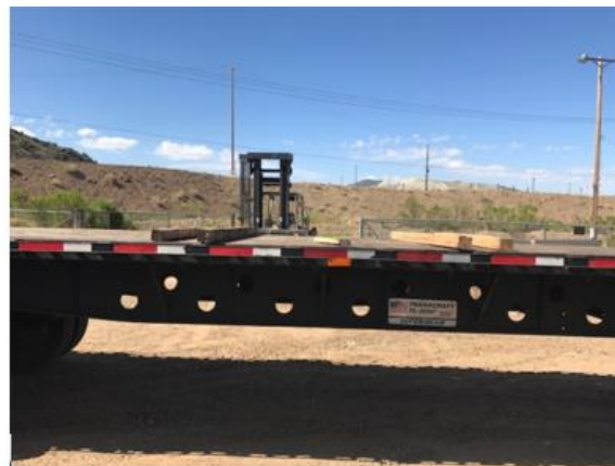
Picture 2: Actual cribbing spacing. The cable reels were setting on the wood 4x4's and were not in contact with flatbed.
