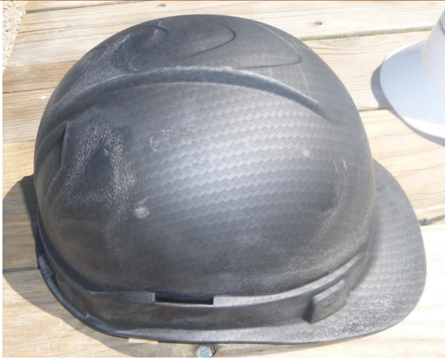
View of deterioration of hard hat
