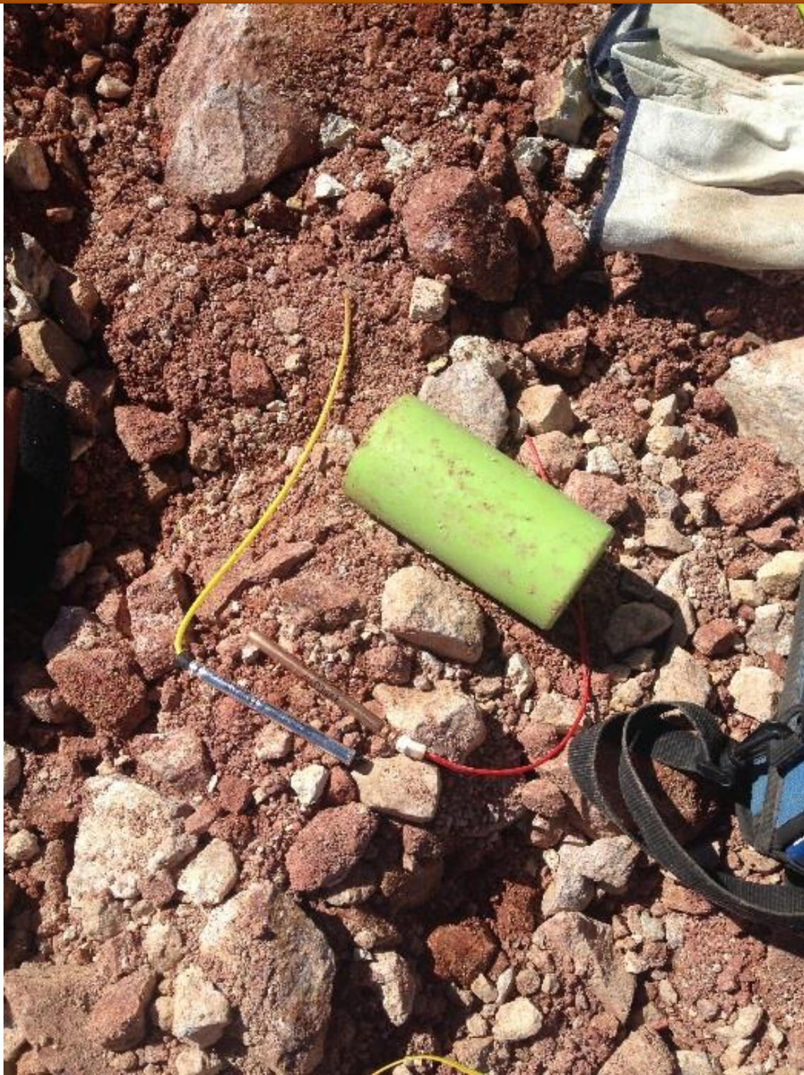
Recovered Booster with i-Kon Detonator and Non-Electric Detonator removed
