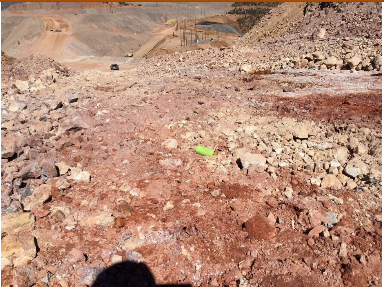
Booster found in work area
