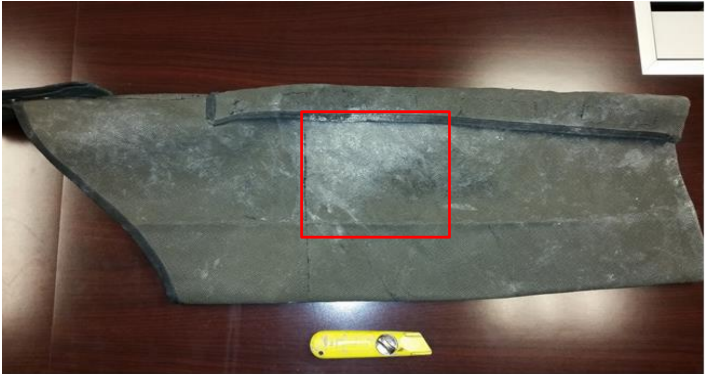
Chaps worn backwards, this minimized the cut resistance area to a single layer.
