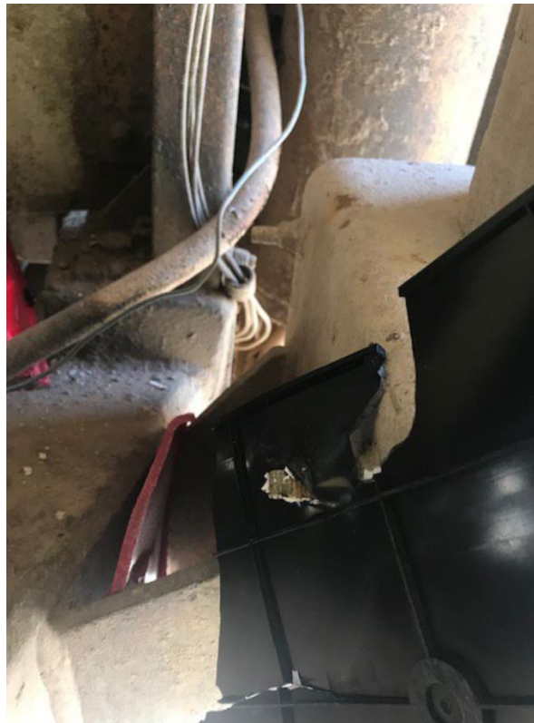
Back panel casing impaled during explosion.
