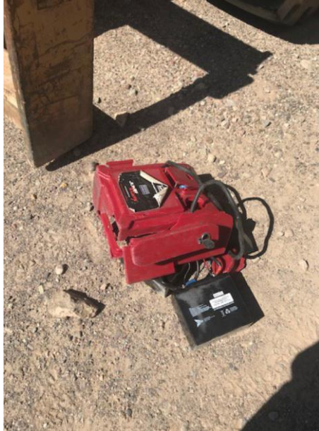
Damage to the jump starter pack (left) and positive grounding cable.
