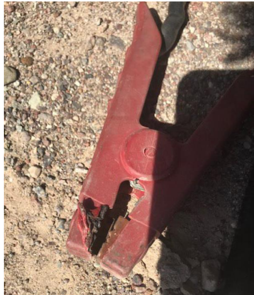
Damage to the jump starter pack (left) and positive grounding cable.
